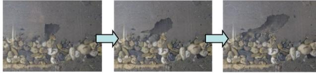
The « **Contact Erosion Test** » or CET is aimed at reproducing this erosion phenomenon in the laboratory.
