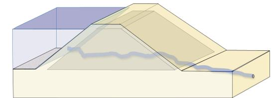
« **Erosion risk assessments and Erosion Tests** »
